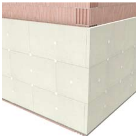
Fixing with a continuous band of glue and central points
